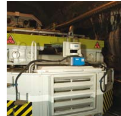
ABOVE CENTRE: Rear navigation scanner along with the deposition hole scanner, which measures the position of the deposition hole in relation to the machine
